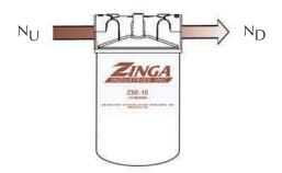
$\beta_{x} = \frac{N_{U}}{N_{D}}$  where x = size of particles in microns (µ) Efficiency<sub>x</sub> = 100 (1 -  $\frac{1}{\beta_{x}}$ )
